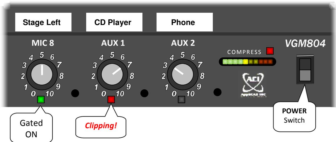
**Gain** controls – adjust as needed for good listening levels. You can apply labels on a blank panel above or below your mixer (as shown above) to describe their actual use. Depending on the microphones and their placement, about halfway up should provide good usable level. If needed, adjust the presets (see the previous page). The gating and compression features mean you'll do less knob-turning than would be needed with non-automatic mixers.
