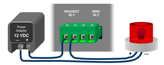
Wire the relay contacts directly in series with a low voltage power source and a signaling device, as shown above. The green connector unplugs from the Telephone Interface should you prefer to wire it separately. Pull straight out to unplug.
