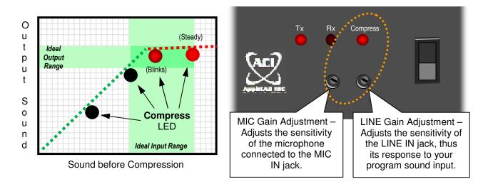
**MIC Gain Adjustment** – Set up your microphone as used normally. Have someone speak (reading a book works well) at a typical distance from the mic. Watch the **Compress** LED:
