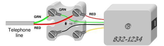
If your wiring uses two-pair cables, the four colors are red, green, yellow, and black. Wire each of the two pairs to its own jack as shown below:
