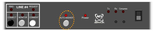
**Select Auto Answer** – Press the **AUTO ANSWER** button. Its LED illuminates. In this mode, the *TIF-401* automatically connects to ringing lines. When in Auto Answer mode, the monitor feature defaults to OFF (you can still select a line to monitor, but it won't automatically switch to the ringing line as before). To cancel Auto Answer, just press its button again.
