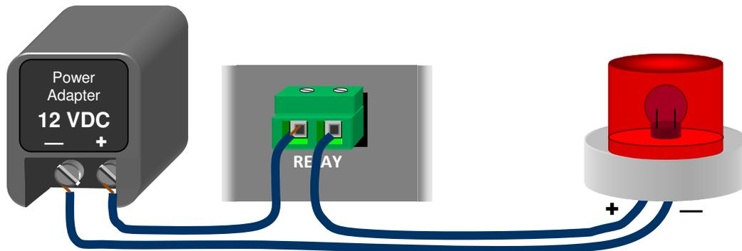
Wire the relay contacts directly in series with a **low voltage** power source and a signaling device, as shown above. The green connector unplugs from the Telephone Interface should you prefer to wire it separately. Pull straight out to unplug.
