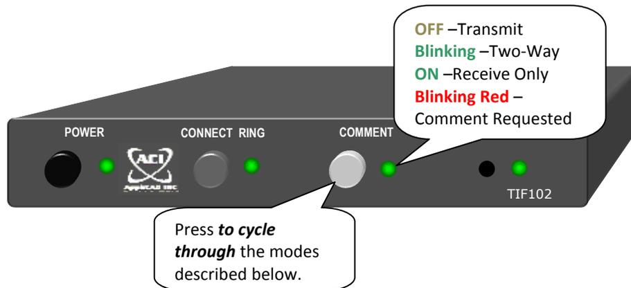
**Preparation** – Have a mic from your sound system handy, and turn up that channel just enough so you can hear yourself when you speak into it. Find the mixer input to which you connected the *TIF-102*'s LINE OUT, and set its control to a low level. Have an assistant call into your line, and press **CONNECT** to connect this caller as you did before. The **CONNECT** LED lights **green**.
