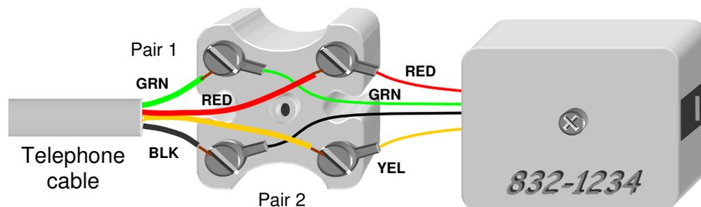
**Tip** – After wiring your phone jack, plug in a telephone and check for dial tone. Then use that phone to call a nearby cell phone -- its Caller ID display identifies your line's telephone number. Label your jack with its number as shown.
