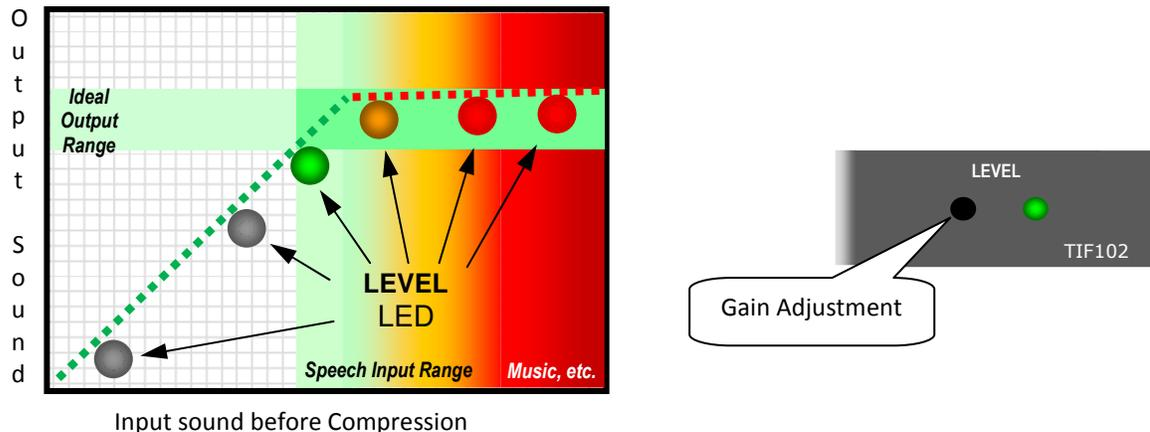
**To Adjust** – Set up your sound system with its most-used microphone. While someone speaks into this mic (reading a book works well), adjust your sound system’s volume for good auditorium listening. Then, watch the **LEVEL LED** at your Telephone Interface:
